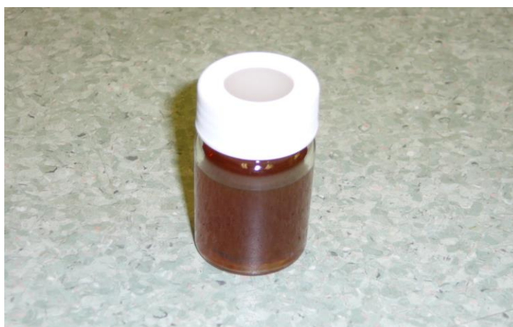
Figure 3: crude oil from dirty waste plastics
